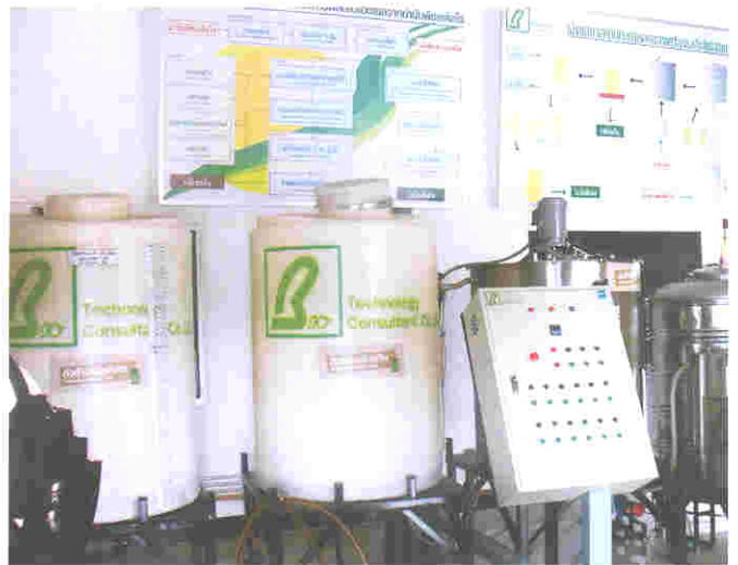
These extraction tanks at Tesco are used to convert used vegetable oil to bio-diesel as recycled energy
