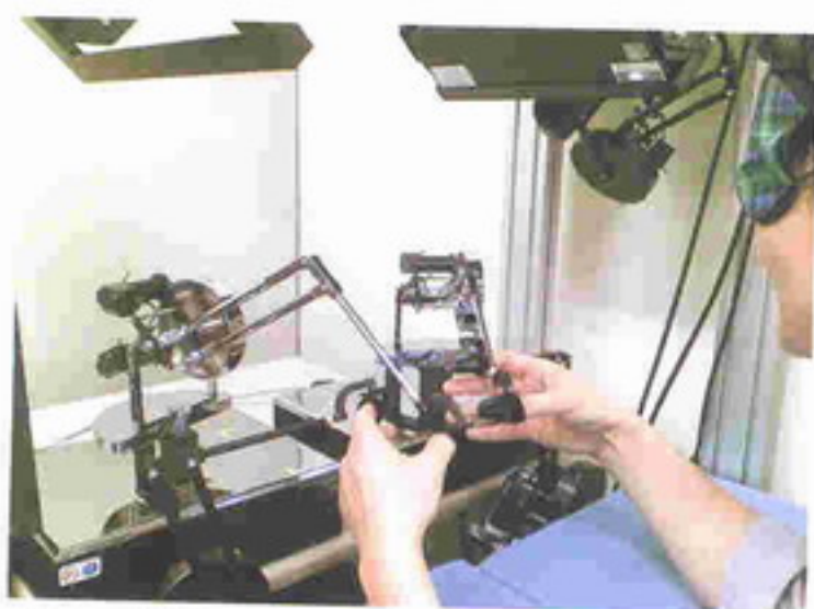
Figure 6: Virtual object shape perception experiment by haptic presentation to multiple fingers of both hands
